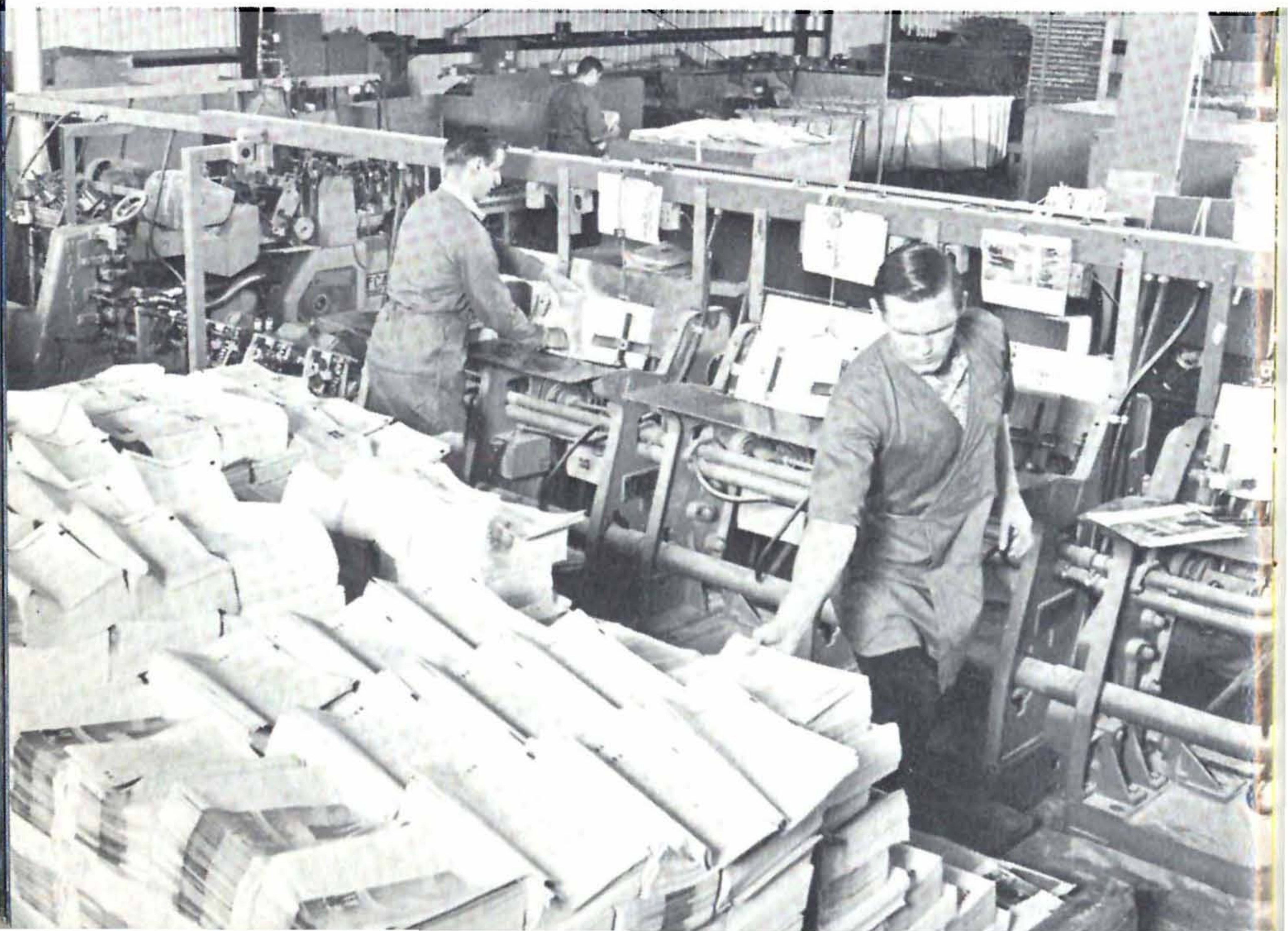
Above, one of the Miehle-Goss 4-color web-fed offset presses, Pasadena plant of Ambassador College Press. Below, one of two large McCain binderies — puts various signatures of magazines together, staples, binds, trims, turning out completed magazines at rapid speed.
